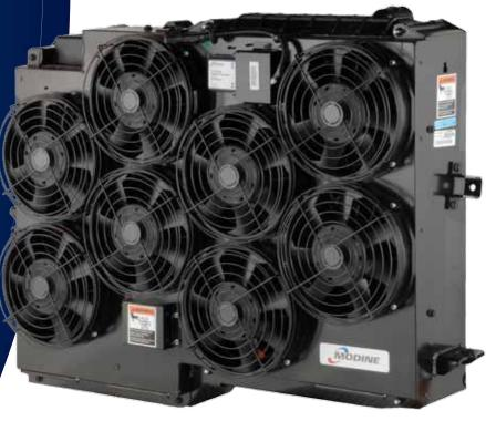
Our new Advanced Cooling System uses the latest brushless electric fan technology to help transit bus systems meet EPA clean air requirements.
