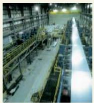
hydraulic controls to adjust thickness and flatness. After leaving the hot-rolling mill, the steel is wound into coils ready for shipment, or for additional processing into cold-rolled sheet, cold-rolled galvanized, or hot-rolled galvanized value-added products.
