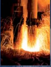
FROM THE COVER: Cascading electric sparks surround giant, glowing graphite electrodes as they bore into steel scrap at SDI's melt shop at Butler, Indiana. To start the melting process, 65 megawatts of power are applied.
