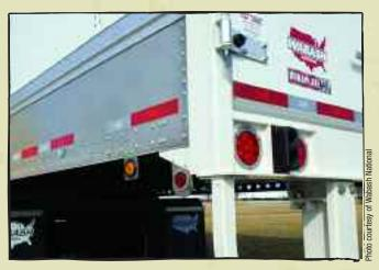
**ABOVE, RIGHT** A finished DuraPlate® HD trailer shows the square pattern of exterior bolts along the side of the trailer, the bolts fastening the side of the trailer to the crossmembers of the undercarriage. Some of the vans that Wabash National builds employ outer skins made of steel. Steel Dynamics is a supplier of painted, cold-rolled galvanized steel for this purpose.
