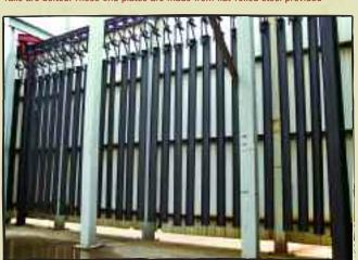
by SDI's Flat Roll Division. **BELOW, LEFT** Crossmembers hang on a conveyor system to cool after being submerged in a bath of hot paraffin to coat them for corrosion protection. **BELOW, RIGHT** Stacked and banded bundles of finished trailer beams are marshaled in preparation for shipment to a Wabash National plant.
