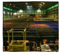
In 2006, the cooling bed at the Columbia City structural mill was extended 80 feet to handle wide-flange beams and rail sections up to 320 feet in length.
