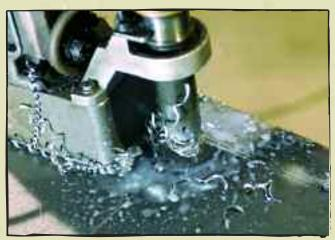
will fasten a baseplate to it. **BELOW, LEFT** Baseplates for columns are drilled. **BELOW, RIGHT** A Helgeson worker punches connection holes in beams.
