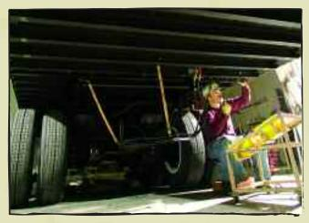
**ABOVE, LEFT** The underside of a finished trailer illustrates the large number of crossmembers used to support an oak floor and the trailer's payload. Once trailer beams are delivered to the Wabash National plant and welded to long rails to form the trailer chassis, the side rails, sides, roof, doors, and mechanical components are added to finish a trailer.
