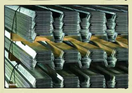
New Millennium Building Systems produces two types of steel products, both used in the construction of non-residential buildings. One type is fabricated joists, trusses, and girders used to support a building's roof and floors. The other type is decking, which is applied over the joists to serve as a base for the floor or roofing.
